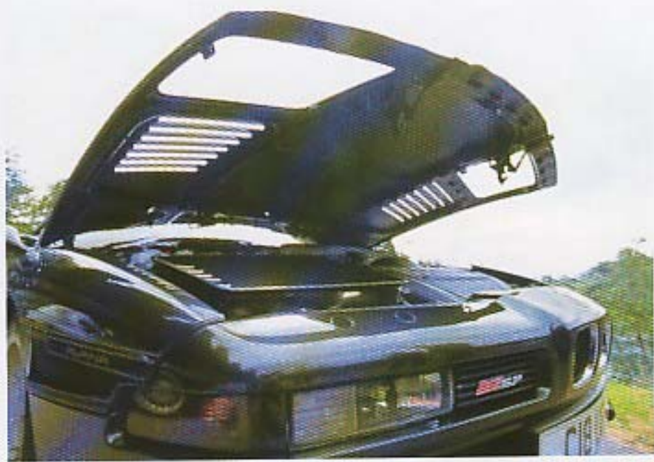
The dramatically ducted Alpina bonnet is carbon fibre over the original steel frame.
